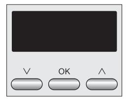
Operate the display with the  $\vee$ , **OK**, and  $\wedge$  buttons.
